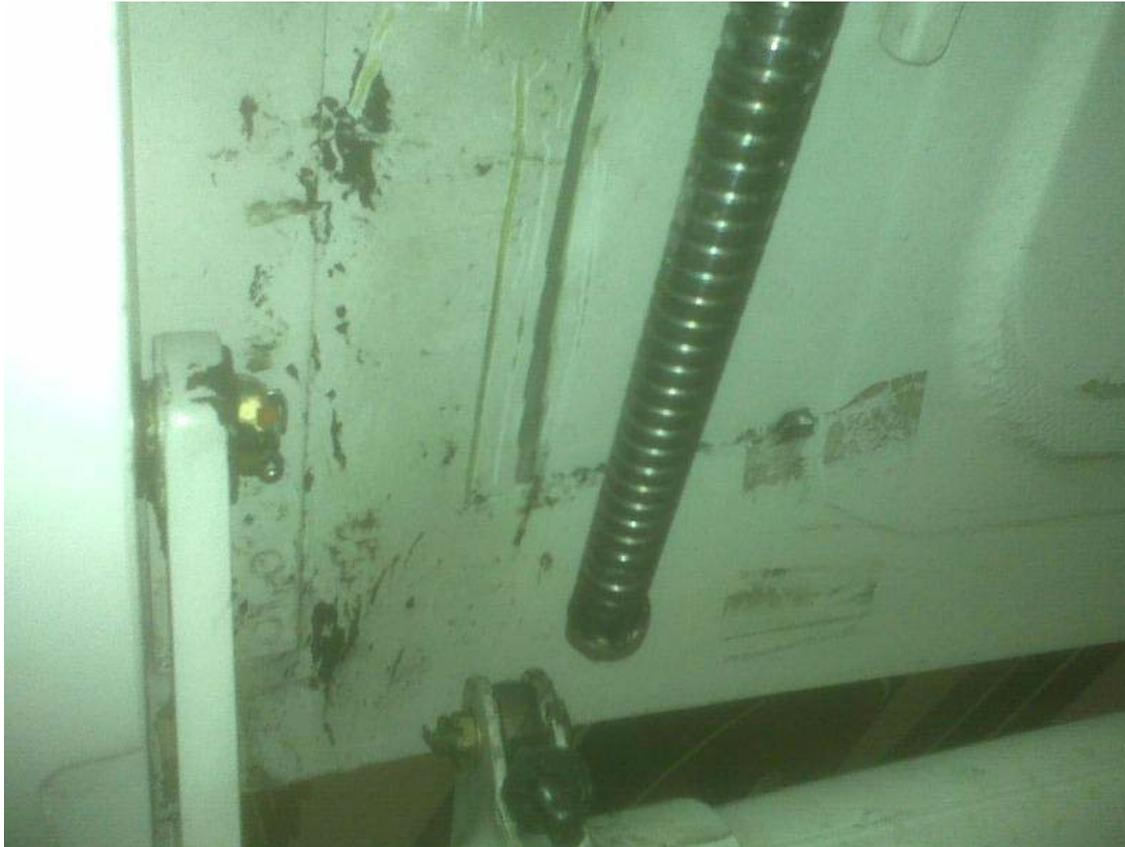
Cessna CE750 Disconnected Flap Linkage, ATA 2750
